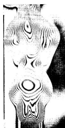
Fig. 13. RBI visualization of a premixed turbulent flame ( \phi=1.6 , Re=1350 , Ri=1 , I=3.2 ).
