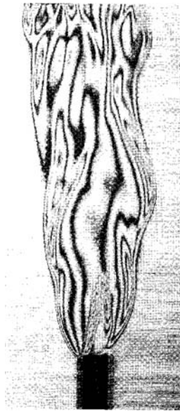
Fig. 15. SI visualization of a premixed flame in lift-off condition ( \phi=1.5 , Re=2315 , Ri=0.06 , l=11 ).
