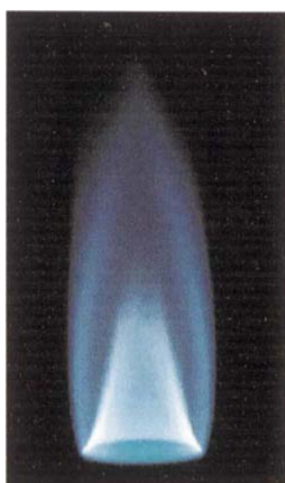
Fig. 12. Direct photograph of a turbulent flame ( \phi=1.6 , Re=1350 , Ri=1 , I=3.2 ).
